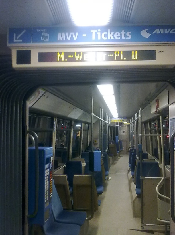
Illustration 9: Over-fading of information due to the direct ceiling lighting which is too intense
