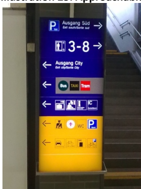
Illustration 24: Good readability due to backlighting as well as different colors for different functions
